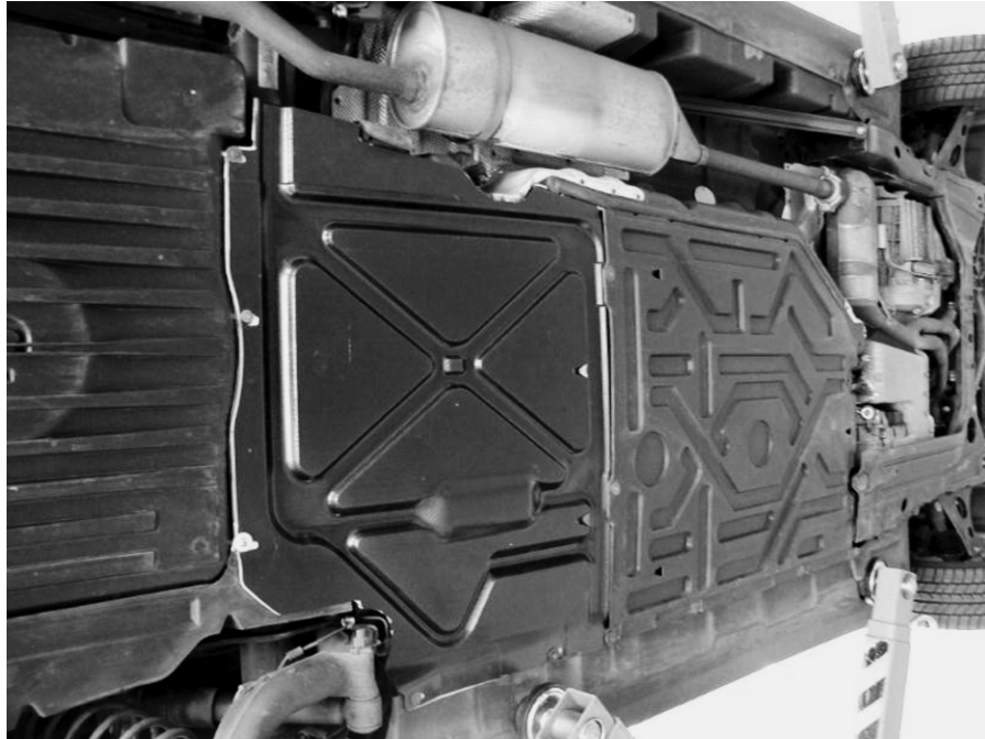
Fig. 11. On vehicle installation of hot compacted PP undertray (Picture by kind permission of BP AMOCO.).
